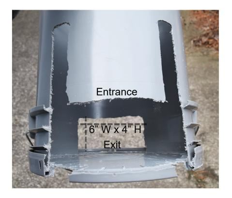
9. Attach the 5-gal lid to the bottom of the bucket (the stage) and mark where the guide boards will be inserted. Cut away to the center portion of the lid. Also, remove the lip in the entrance (between the boards) with a Dremel or hacksaw.
