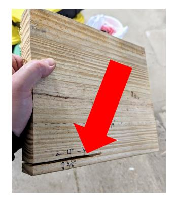
1. Remove bottom (will become top of camera trap) using a Dremel with circle cutter (model 678).
