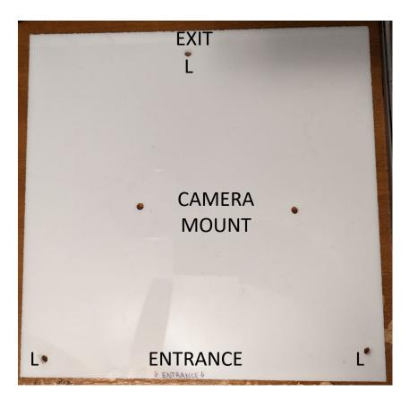
13. Center the acrylic over the bucket, making sure it is nearly flush with the bucket on the front entrance side that will be flush with the fence. On the acrylic, mark where the outer holes are located for the two front brackets; mark the inner hole for the bracket over the exit. Once the holes are marked, use a 1/4" bit to drill the holes.
