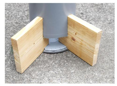
11. Use 6 machine screws and nuts to attach the "L" brackets to the (now) top of the bucket. Bucket is complete!
