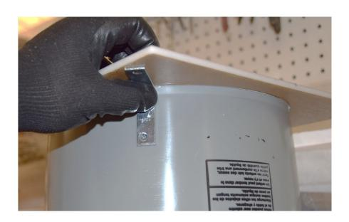
4. Drill the holes for the 3 "L" brackets (total of 6 holes). Note: the brackets are not evenly spaced on the bucket, and the two closest ones make up the *front* entrance of the camera trap.
